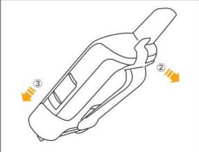
1.Install the back clip: As shown in Figure 1, insert the back clip into the fuselage from bottom to top until the top buckle of the back clip engages with the groove on the top of the fuselage.
