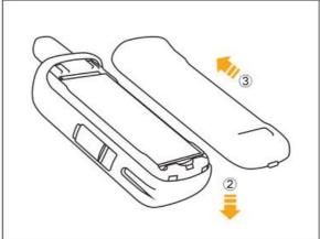
As shown in Figure 1, place the battery into the battery compartment. The positive and negative directions of the battery correspond to the markings in the battery compartment. As shown in Figures 2 and 3, close the battery back cover and push it upward until the battery cover is fixed.
